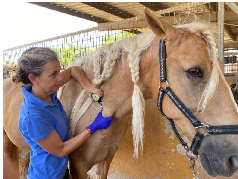
Figure 2. Maria Calatayud-Bonilla measuring pressure pain threshold with an algometer at the distal portion of the brachiocephalic muscle.
